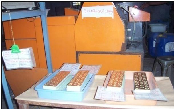
Fig.2 Kanban card system to regulate material flow
